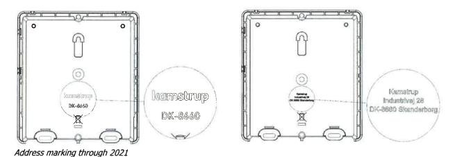
CE marking and the supplementary metrology marking System designation (No. of the EU-type Examination Certificate) Type, production year and serial number Temperature limits ( $\theta_{min}$  ...  $\theta_{max}$ ) Differential temperature limits ( $\Delta\Theta_{min}$  ...  $\Delta\Theta_{max}$ )
