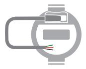
On the cable connected to the wired interface, the pulse output is between the black and the red wire.
